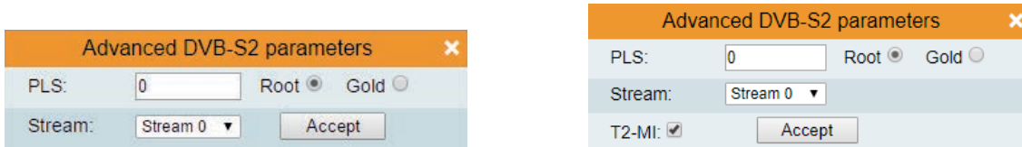
Figure 14. "Advanced DVB-S2 parameters" tables (T2-MI deencapsulation is supported only in M.1 version)
